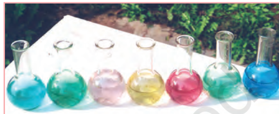
Fig. 8.5: Colours of some of the first row transition metal ions in aqueous solutions. From left to right: V^{4+} , V^{3+} , Mn^{2+} , Fe^{3+} , Co^{2+} , Ni^{2+} and Cu^{2+} .
