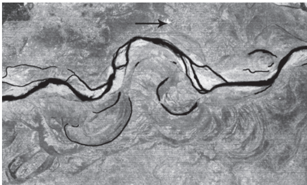
Figure 7.7 : A satellite scene showing meandering Burhi Gandak river near Muzaffarpur, Bihar, showing a number of oxbow lakes and cut-offs
