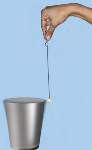
Fig. 13.17 : Thermocol ball touching the vibrating glass tumbler
