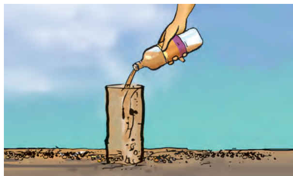
Fig. 9.5 Measuring rate of percolation
